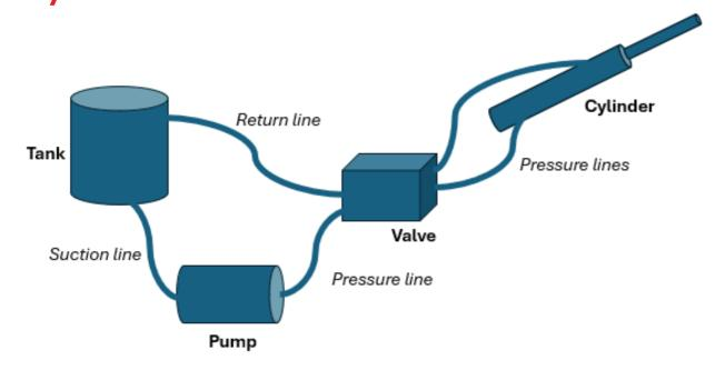
In the most basic hydraulic system, there will be a cylinder, or sometimes a hydraulic motor, that is providing motion. The power to drive this comes from the hydraulic pump, which is electrically powered.
